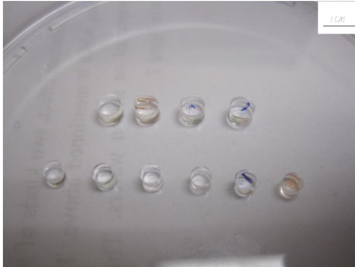
Figure 6.b. Cylindrical PDMS network samples for compression tests.
